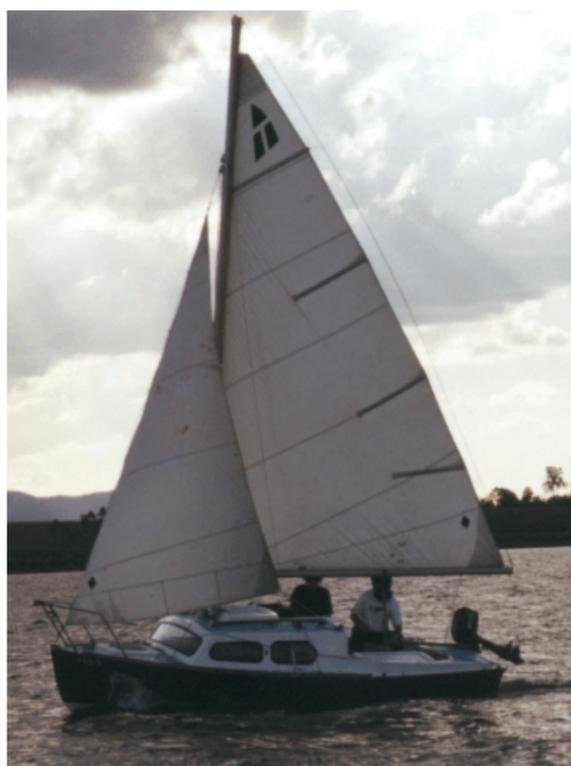
Here is a clean-lined conventional sheered little yacht with a well-designed cabin top. Besides ample space for a party out daysailing there are two permanent bunks for week-end cruising. She sails efficiently under a small, easily handled sail area and drives cleanly under power.
