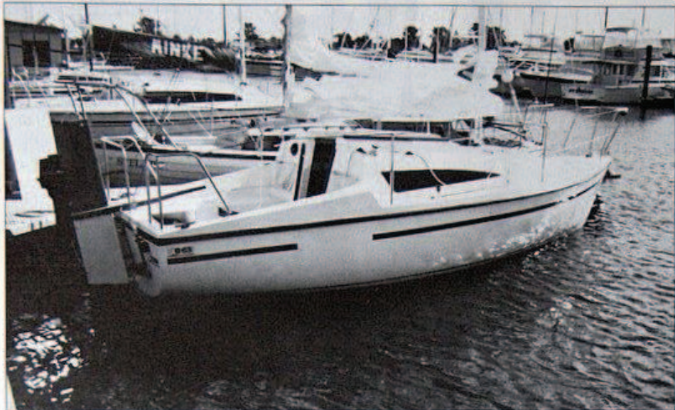
Deck-line has been raised; profile eye pleasing in deck-mould re-design.
