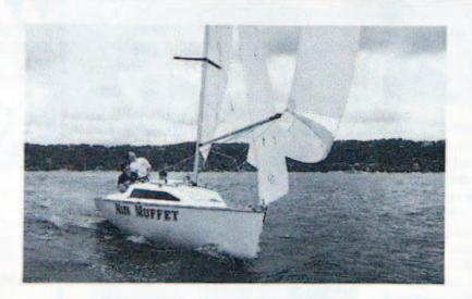
WITH the combination of light weight, extremely slippery hull shape and a skiff-style rig, the Aussie designed and built Spider 22 has long been the uncrowned champ of the pocket-rocket market and a true giant-killer.
