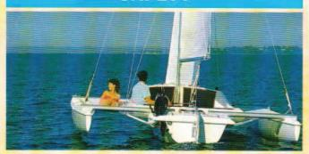
With over a million sailing miles achieved by Farrier trailerable trimarans the seaworthiness of the OSTAC TRAMP is guaranteed. Her enormous beam gives unmatched stability and foam buoyancy together with a total of seven major separate watertight compartments make her virtually unsinkable.
