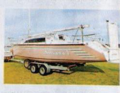
strikes a nice balance between the outright performance of the modern ultralight TSs, such as the Ross 780, Young Rockets and Spider 28, and the needs of comfortable cruising. It just sneaks in under the boundary for light displacement while still retaining good interior room and comfort through a relatively high freeboard and generous sized coach house.
