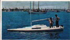
Here is a test of the boat's foam flotation. We drilled a 1½° hole in the hull bottom, opening the boat to the sea. This is how it ended up when full. It won't sail fast this way, but if beats swimming.
