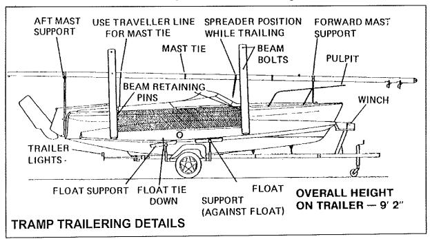
about 9' 2" As a result, care should be taken to watch for low clearance bridges, overhanging tree limbs, etc. Should it be necessary to take the boat under a low obstacle, the height can be reduced by unfolding the floats. Although the extended floats will increase the beam width, the height can be significantly reduced.
