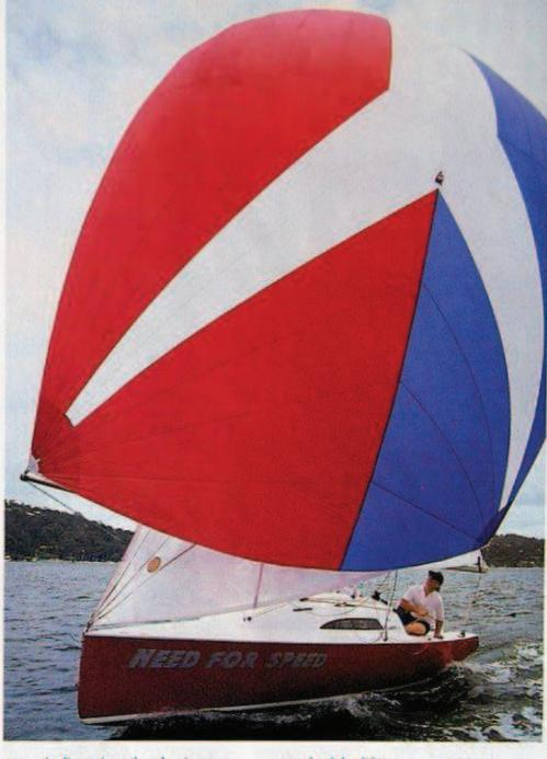
owner's discretion, the class' onedesign aspect only covering the hull, mast and foils. Kerli has opted for Ronstan gear in his fitout, including the stylish new cam cleats and low-profile, recirculating-ball mainsheet traveller. His previous catamaran sailing experience is born out in his choice of mainsheet system, very Hobie 16, and sails, from former Tornado champion Chris Cairns.
