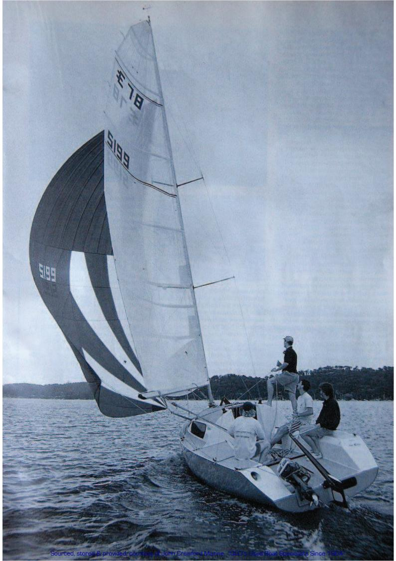
skiff-type TS hulls and this plays a major role in the boat's performance. By keeping the bow section relatively "full" compared to the mid and stern, the bows do not dig in when the hull heels.
