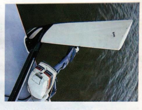
daggerboard. It enhances the sense of airiness when the board is lowered, and there's no way water can escape into the cabin. The 400kg fin is raised with a simple trailer winch fitted with Spectra rope. Mounted on the centre case in the cabin, it works beautifully considering the weight of the board.
