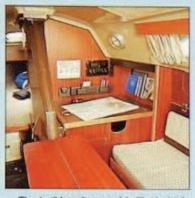
The bulkhead assembly illustrated giving good and private separation within the accommodation, also the galley area which converts into a chart table when required.
