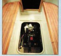
On both the Dehlya 22 and Dehlya 25 class yachts secure stowage is provided under the cockpit sole for an outboard motor. On the Dehlya 25 an alternative inboard auxiliary marine diesel engine can be fitted if preferred.
