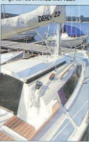
Halyards and quick reef line to the main sail lead aft to the security of the cockpit through stoppers (rope clutches) to winches.
