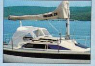
The folding pramhood so convenient in harbour or under sail improves standing headroom and helps to maintain a dry and well ventilated interior in all weather conditions.
