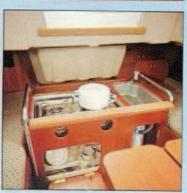
Galley unit when stowed under the bridge deck.
