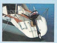
The Dehlya 22 performs well under power using a light weight 4/6 H.P. outboard motor mounted on our quick raising and lowering system to reduce drag under sail – also convenient when the yacht is being launched and recovered to the road trailer.
