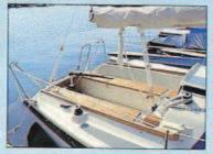
With our kit (Packet) No. 4 the cockpit seats, cockpit sole and combings can be trimmed with Teak.
