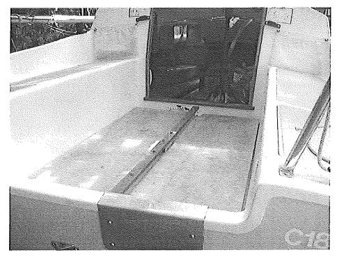
Then flip the sheet of ply over, so the bracing strip is on the bottom. Those gaps "strategically placed" in the lengths of cypress allow you to feed the support strips through, so they won't slide around (though this shouldn't be a problem). Note that this process is a bit awkward. If you didn't want the bracing strip, you would avoid having to flip the ply sheet.
